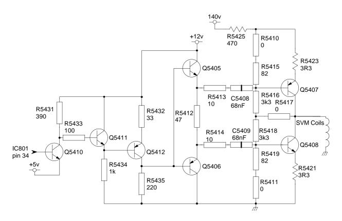
The signal that is used to control this circuit is derived from IC801 pin 34 and the amount of correction can be adjusted by the end user via the picture menu.
