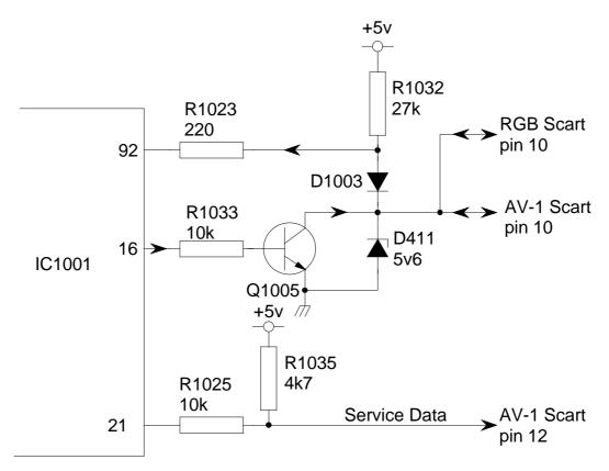
Data from the CTV to VCR is from IC1001 pin 16 via Q1005 and is outputted from pin 10 either AV-1 or RGB SCART sockets. Data from VCR is from the same SCART connection but this time it is fed into IC1001 pin 92 via D1003. D411 provides protection from excess voltage being applied to the SCART sockets.
