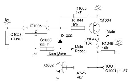
Its function is to remove the line drive by turning on Q607, thus placing short between the horizontal drive signal and ground, at the same time this HOUT pulse will cause the audio mute circuits to activate, preventing any noise from the speakers.
