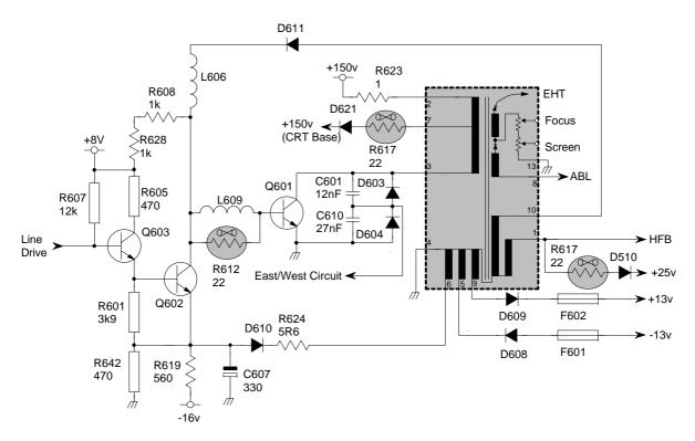
With this type of driver circuit, it is essential that the circuit is started softly, otherwise transient pulses can damage the line output transistor. This is achieved by doubling the horizontal drive frequency; which effectively reduces Q601 on time, until the run voltage has been established.
