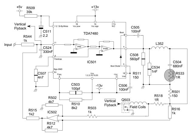
The PWM signal from pin 4 of the IC, is passed through a low pass filter (L352 and C504) producing a ramp signal at the field deflection coils. This ramp waveform will vary between +13v when the scan is at the top of the screen decreasing to -13v when the scan has reached the bottom of the screen. The field scan coils are returned to ground via Q503. Q503 is turned on during the vertical scan period and turn off during vertical fly-back.
