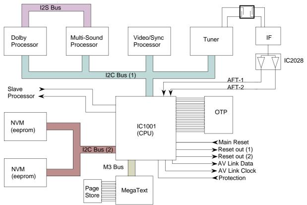
**PARALLEL BUS** Communication between the CPU and the OTProm (one time programmable read only memory). This device contains the software (operating system)
