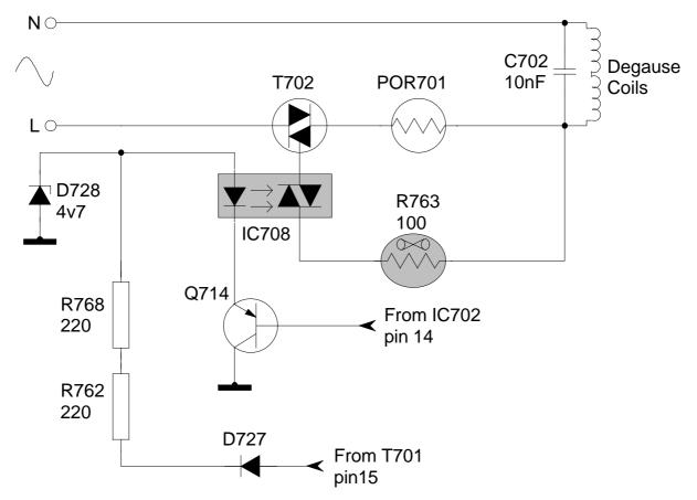
Current will continue to flow through the degauss coils until either the PTC (POR701) has increased in value sufficiently to cut off the current flow, or IC702 pin 14 goes high, turning of Q714, preventing current flow through IC708, turning the triac T702 off.
